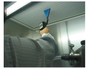
Validation service ULPA/HEPA Filter Integrity (DOP) Test
